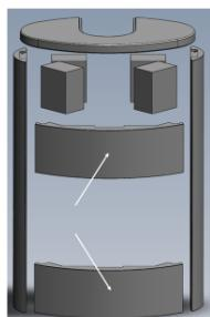
**3.** The two front stones are identical, so it does not matter which stone goes at the bottom or top.
