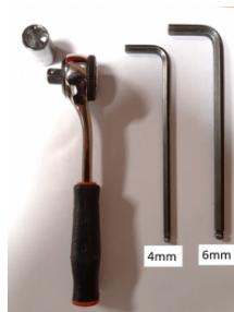
**4.** For mounting, use a 4mm and a 6mm Allen key. A little socket spanner and a 10mm top.
