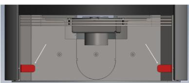
**5. Bottom stone:** Fit the angle irons provided inside the fuel compartment. Mount and adjust the angles so the stones are in place and are flush with the edges of the stove.
