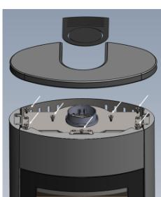
**10. Top stone:** The top stone should be loosely placed on the top, with the prepared holes matching the mounted threaded studs with fitted nuts.
